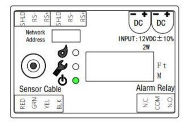
In normal working state (no leakage), the LCD screen is in the state of "four horizontal lines flashing", as shown in the figure below, otherwise, the fault indicator light flashes orange, please check whether the sensing line is connected correctly;
